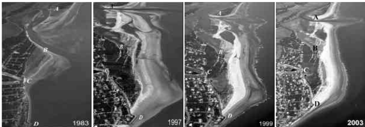
FIGURE 7. Oblique aerial photographs at low tide, looking updrift from Seabrook Island to Captain Sams Inlet and Kiawah Island. Point A marks the excavated inlet. Point B is the terminus of the original inlet. The area from Point C to Point D is armored. The reach downdrift of Point D (out of the photographs) is the margin of North Edisto Inlet, an adjacent littoral compartment.
