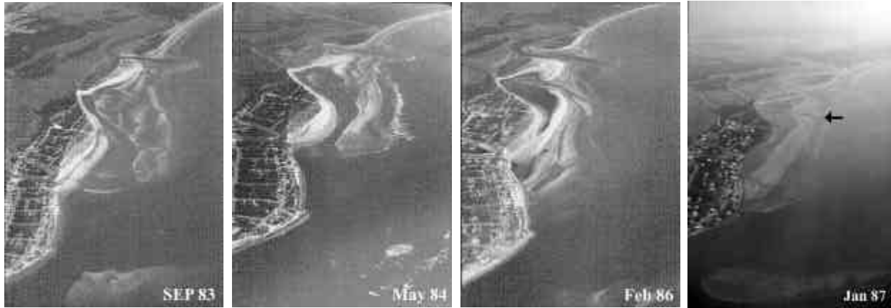
FIGURE 3. Morphological changes at Captain Sams Inlet after inlet relocation in March 1983. Views looking north at low tide. Slough (arrow) drained a new lagoon formed by accreting ridges.
